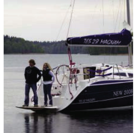
One of the neatest features is the easy-to-use lifting swim platform that folds up to close the back of the cockpit.
